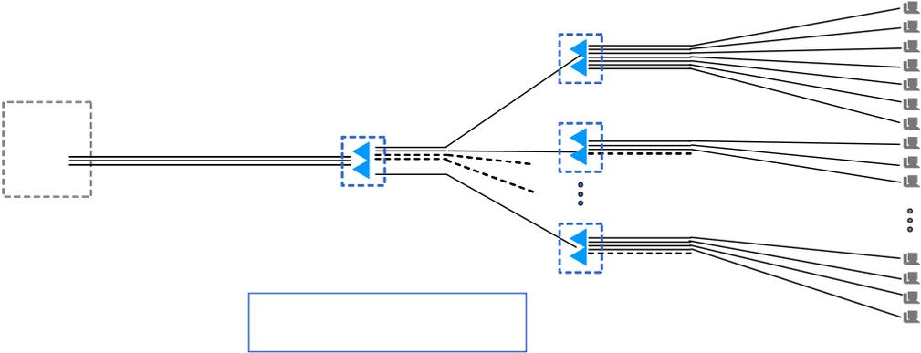
PON operators need to achieve a balance between optimising investment costs (optimising occupancy on the branches, but with a need for regular work to be performed at the points of flexibility where the splitters are located) and optimising operating costs (limiting the amount of work done at the flexibility points, which implies a lower rate of occupancy on the branches).
