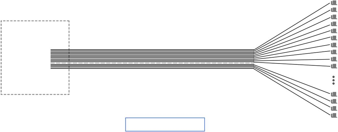
In addition, the installation of optical distributors can require a substantial investment as there are, in principle, as many optical fibres arriving at this concentration point as there are households located in the ODF’s service area (several thousand). Although the optical fibre takes much less space than copper telephone lines, the ODFs can nevertheless occupy a sizeable area.
