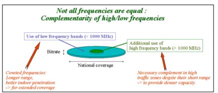
1 GHz to be made available. These frequencies have better physical radio propagation qualities, enabling a longer range and better indoor penetration. This is why the low frequency bands, i.e. below 1000 MHz, are so highly coveted. They are well suited to achieving extended nationwide coverage for mobile services under reasonable economic conditions, along with indoor penetration equivalent to that of existing networks.
